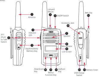
The table that follows is a numbered description of the parts of the TX667 radio, as labeled in the diagram above.
